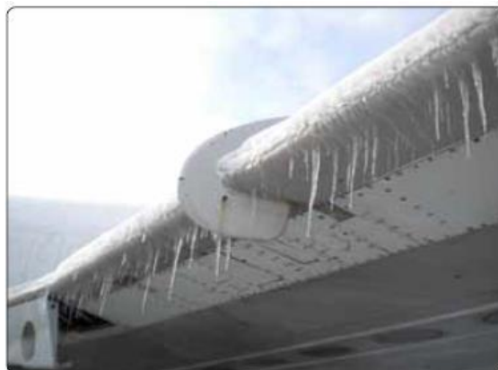
Formation of ice on aircraft leading edge.
