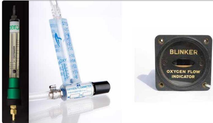
Different flow indicators are used to provide verification that the oxygen system is functioning: continuous-flow, in-line (left); continuous-flow, in-line with valve adjuster (center); and old style demand flow (right).
