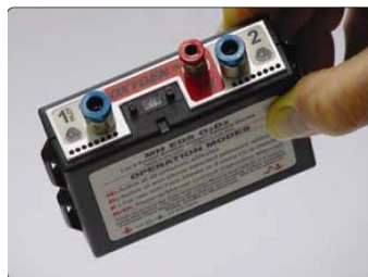
A portable two-person electronic pulse-demand (EPD) oxygen regulating unit.
