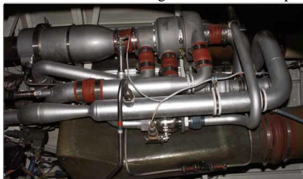
An air cycle air conditioning system used to pressurize the cabin of a business jet
