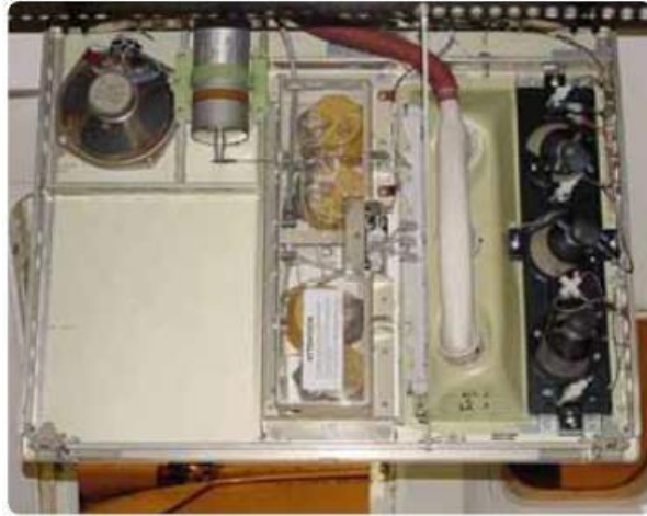
An oxygen generator mounted in place in an overhead passenger service unit of an air transport category aircraft.
